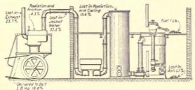
Fig. 258.-Loss in a suction gas-producer plant.\*
